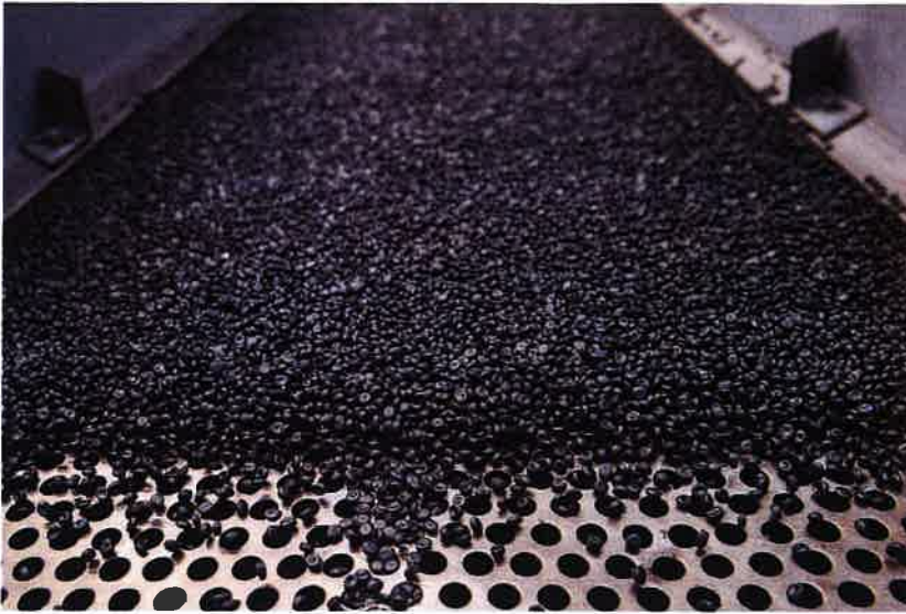
Compound obtained with the upcycling process on the Evorec Plastic Plus line
